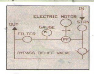
Transfer unit Oil can be easily transferred from an oil drum to the machine reservoir or vice versa.
